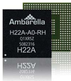
The 14 nm H22A SoC Device
