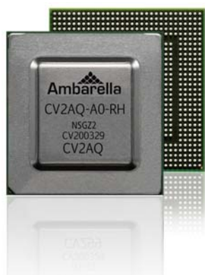
The CV2AQ chip targets automotive sensing camera designs
