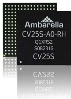
The CV25S chip targets IP camera designs
