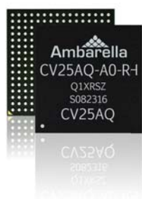
The CV25AQ chip targets automotive sensing camera designs
