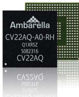
The CV22AQ chip targets automotive sensing camera designs
